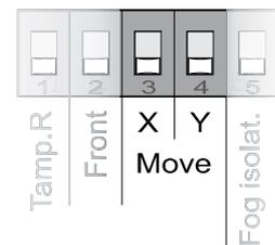
The motion sensitivity is adjustable via two DIP switches [Move] pos. 3 en 4. See also pag. 13.
